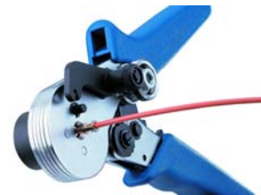
Removal of crimped contact
